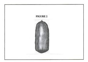
The height of the cavern is approximately 800 feet and has a diameter of approximately 350 feet. The top of the roof is 1410 feet below ground surface (bgs).
